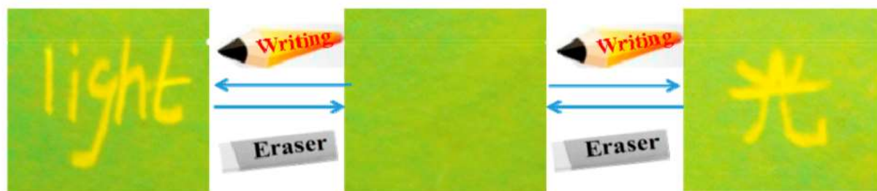
Figure 2. FL spectra of APPTPECN as pristine, grinding and fuming samples (a); Repeated switching of the solid-state fluorescence of APPTPECN (b) by repeated grinding and fuming cycles; (c) Photos of the luminescence writing/erasing process on the APPTPECN-loaded paper under a 365nm UV lamp.
